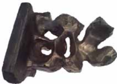
Underside of Modular Vantage Coal Bed Section. Note ports for the gas to flo through.
